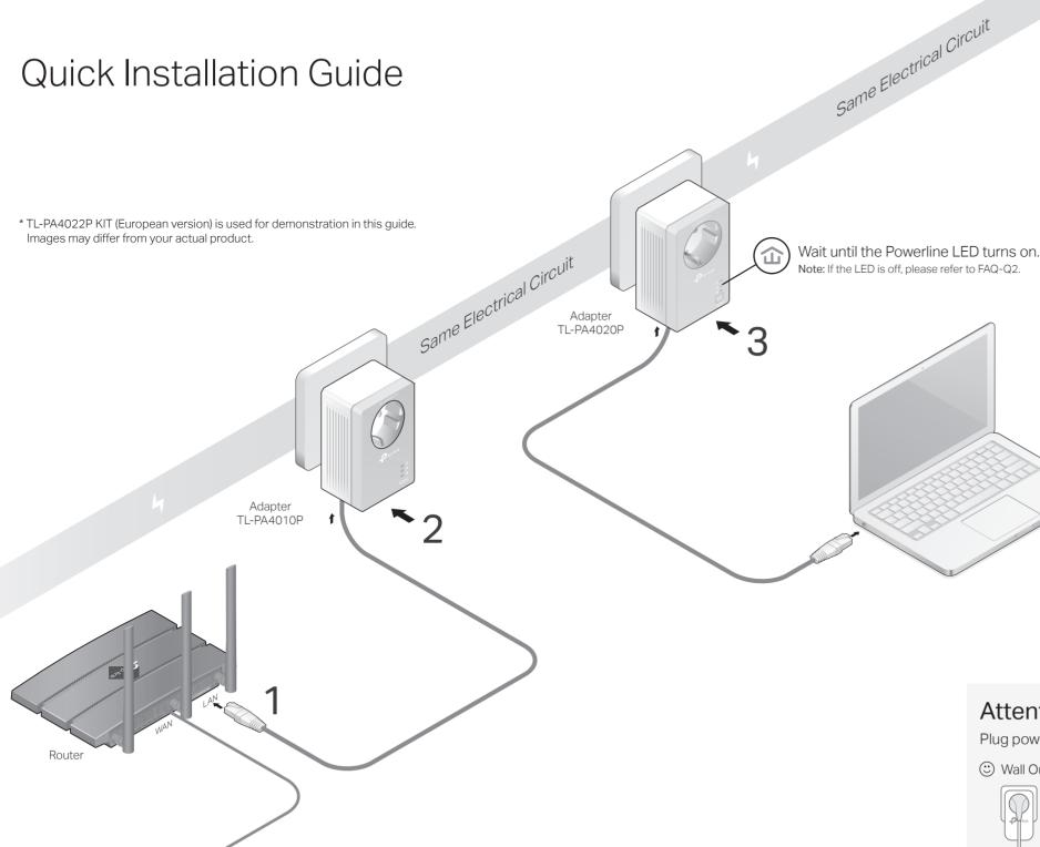
More: To add additional powerline adapters and extenders with the default settings, simply plug them into the wall sockets on the same electrical circuit.
